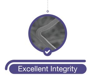
*e*G coating allows the polymer to have excellent coating integrity, even after tortuous-path testing and balloon expansion (seen in scanning electron microscopy<sup>5</sup>).
