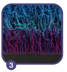
The filament-like structure of the *e*G coating allows interdigitation of the PLGA coating, forming a strong bond.
